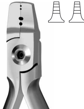
Lingual Arch Plier NE-12-3112 11.5 cm/ 4½" Designed to form double and triple bends in either .030" (0.76 mm) or .036" (0.91 mm) wire for inserting lingual sheaths
