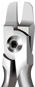
Tweed NE-12-4611 T/C 11.5 cm/ 4½" Rectangular Arch Pliers, Tweed Style Forming plier for square or rectangular wires. The blades are designed to be parallel at .020" ( 0.51 mm ) opening. The working edges are carefully diamond-honed to prevent wire scoring.
